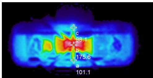
Figure 4. Temperature map just after boiling at 18s of the measurement procedure. The movement of the boiling vapor phase is visible in point a.
