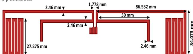
Figure 2. Layout of the proposed dual-band antenna
