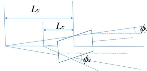
Figure 4. Coordinate system of divergence array transmitter with anisotropic directivity.
