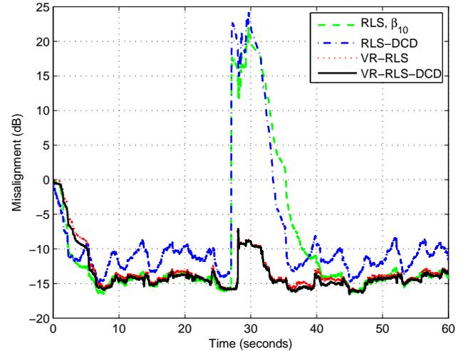
Figure 9. Misalignment of the regularized RLS (using  $\beta_{10}$ ), RLS-DCD, VR-RLS, and VR-RLS-DCD algorithms. The input signal is speech,  $L = 512$ , and ENR = 10 dB. Near-end speech appears between time 27 and 30 seconds (double-talk scenario).
