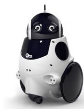
Figure 1. Photography of the robot Qbo Pro Evo without the Asus Xtion Pro Live RGB-D Camera.
