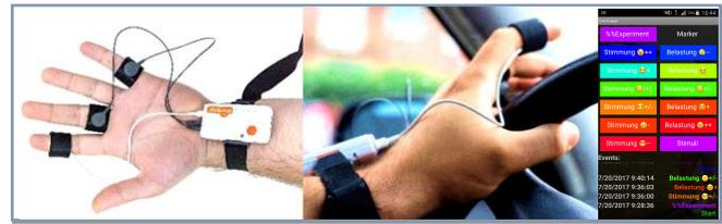
Figure 7. Experimentee with GSR electrodes and PPG fingertip sensor (left and middle); Event logger interface (right).
