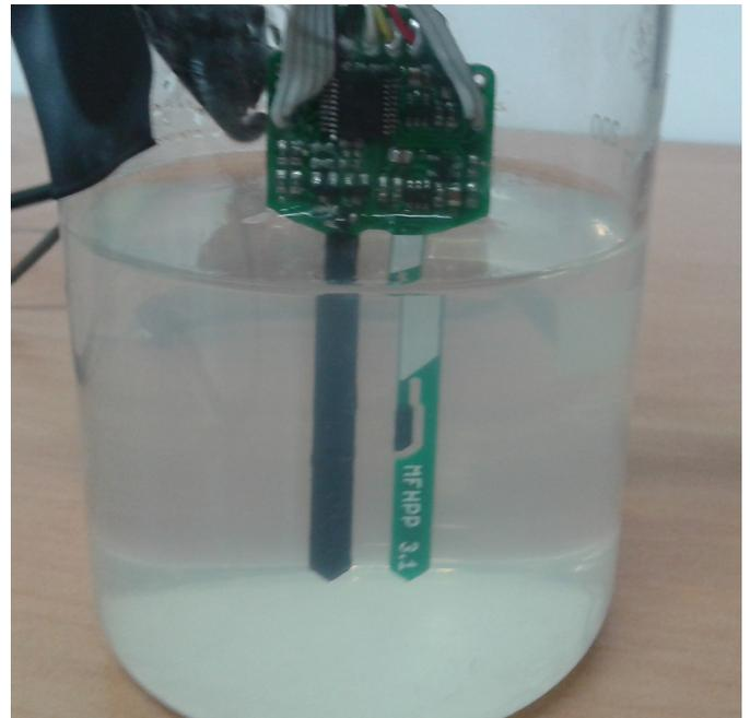
Figure 5. Probe distance calibration in agar solution
