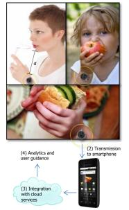
Fig. 1. A high level architecture of the proposed system is shown above. Many different forms of eating can be detected using a smartwatch, provided the appropriate hand is used and the watch is brought close enough to the mouth.
