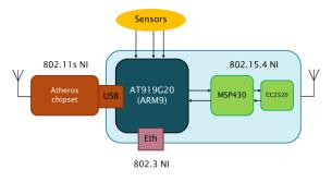
Figure 2. Network node block diagram
