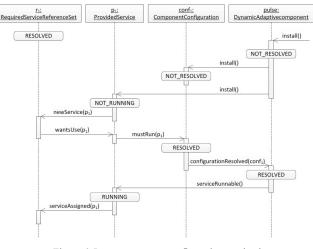
Figure 6. Inter-component configuration mechanism.
