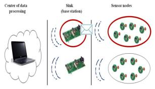
Figure 1. Wireless sensor network architecture
