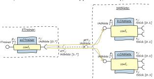
Figure 15. Example for possible assignments of the quantity uses.
