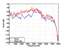
Fig. 3. Frequency distribution of a water swallow vs. silence (noise). This graph reveals that the frequency range between 500 Hz and 1000 Hz is the point of interest.
