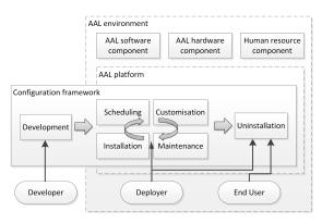
Figure 2. The configuration framework with its stakeholders and their involvement in the configuration phases.
