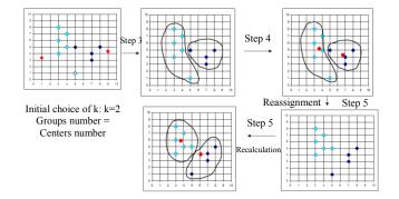
Figure 4. Operating principle of K-means algorithm
