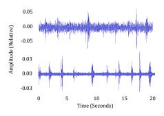
Fig. 4. Post-processing of the audio signal corresponding with water can dramatically improve signal-to-noise ratio. The top shows the original waveform. The bottom shows the waveform after a bandpass filter is applied.
