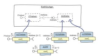
Figure 12. Suitable components for an application configuration.
