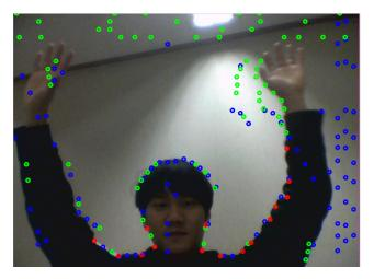
Figure 2. Harris corner detection on a frame in three orthogonal planes, (x,y), (x,t), and (y,t) [red = (x,y), green = (x,t), blue = (y,t)].
