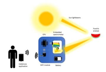
Figure 1. User centric based device for food pesticides monitoring
