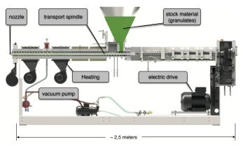
Figure 1. Working principle of an extruder (courtesy: Hans Weber Maschinenfabrik, Kronach, Germany)
