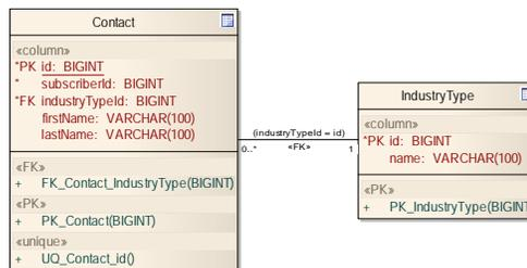
Figure 3. Shared schema for a SaaS application
