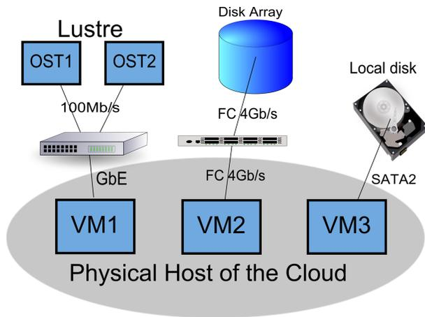
Figure 2. Test environment for storage QoS.
