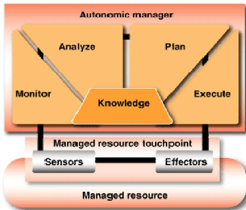
Figure 1. Autonomic loop (or MAPE/MAPE-K loop) [1].
