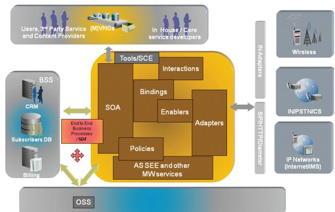
Figure 2 – Blueprint and positioning in a Telco Environment (or generic Service provider environment) of a SDP as Middleware + Telco (in fact communications as this works also on internet for ISPs) functions, capabilities and performances [5].
