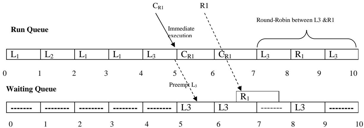
Figure 3. Proposed Scheduling Mechanism for CASE A
