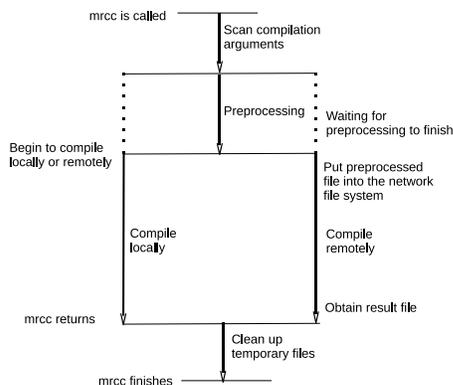
Figure 2. The work flow of mrcc
