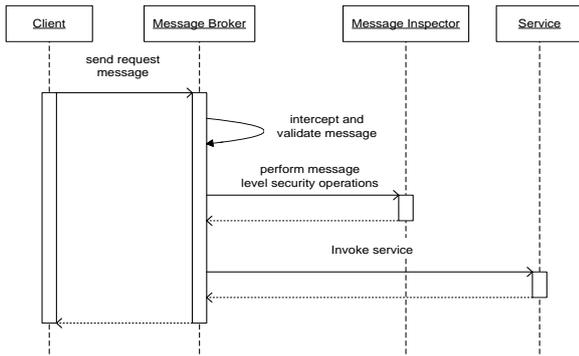
Figure 4. UML sequence diagram – Message Broker component
