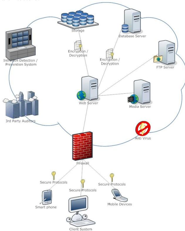
Figure 1. High Level Cloud Storage Architecture.
