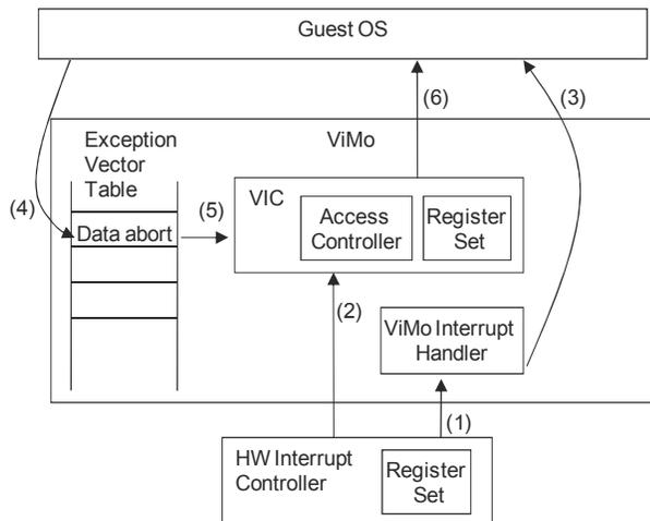
Figure 5. Interrupt Handling
