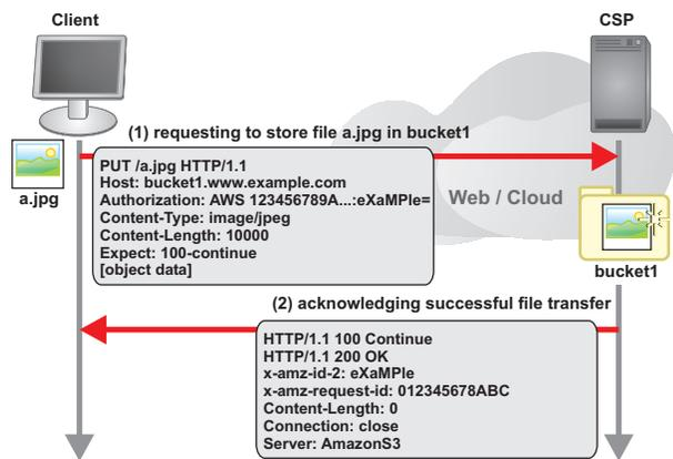
Figure 1. Basic access structure of Amazon S3
