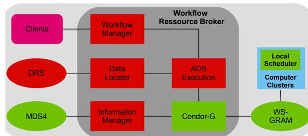
Figure 2. The components of the Workflow Resource Broker.
