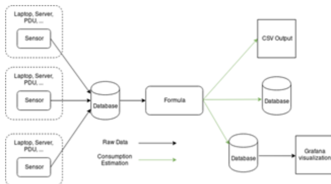
Figure 1. The global architecture of a power meter
