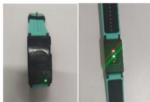
Figure 1. Device used (MAXREFDES103).
