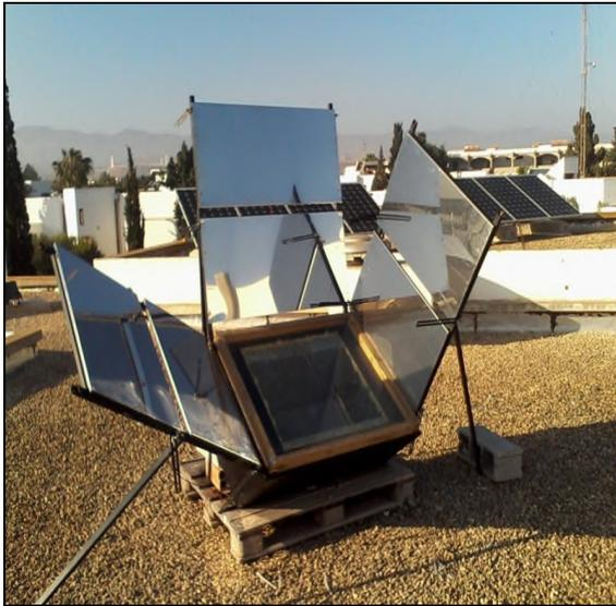
Figure 1. Solar furnace with three external reflectors.
