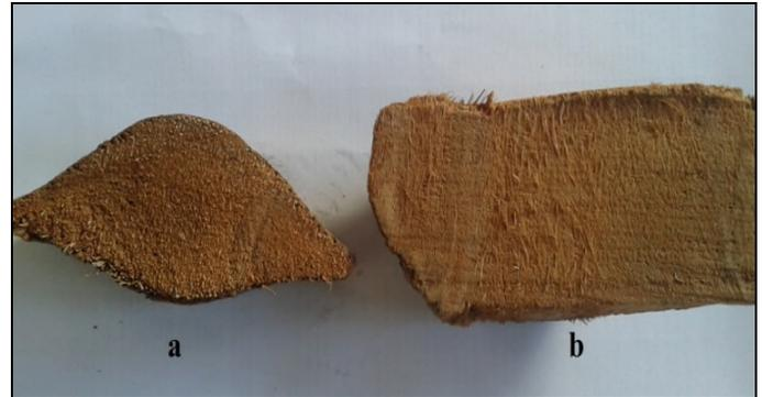
Figure 3. Samples cut out from the petiole (a) petiole sample I longitudinal direction of fibers, (b) in transversal direction of fibers.
