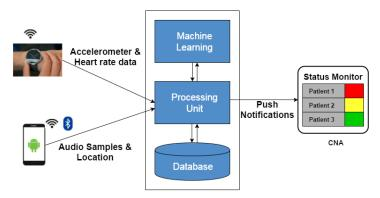
Figure 1. Architecture of the Monitoring System
