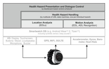
Figure 3: Block diagram of the smartwatch app
