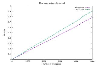
Figure 4. Overhead of Flow Registration
