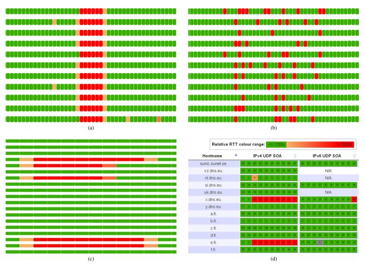
Figure 2. Examples of problem analysis. In (a), (b) and (c) the main matrix is represented, with x-axis (time) and y-axis (anchors) removed to obscure identities. (a) An outage where all anchors had severe problems reaching the server, causing a thick vertical band. (b) Partial denial-of-service attack, shown as a scattered vertical band. (c) Outage affecting a subset of anchors, with solid horizontal rows. (d) Recent measurements by an anchor.
