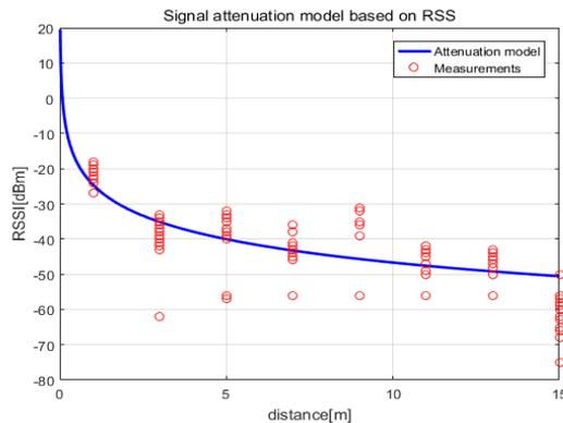
Figure 1. Signal attenuation model for indoor positioning
