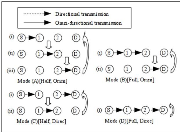
Figure 1. Transmission process for each operation mode [9].
