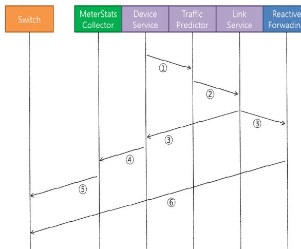
Figure 5. Flowchart of interactions between sub systems
