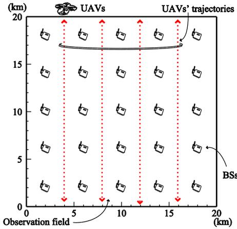
Figure 3. Deployment and trajectory of SNs, BSs, and MBSs (UAVs)
