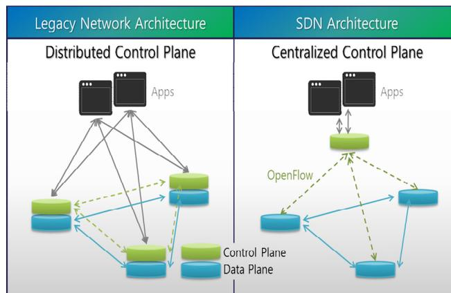
Figure 1. Compare with between legacy and SDN architecture.
