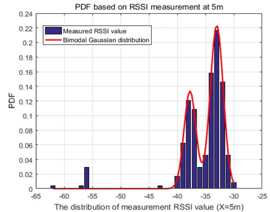
Figure 3. Probability density function of RSSI measurements at 5m
