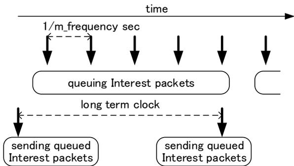
Figure 1. Implementation scheme of coarse-grained clock system.
