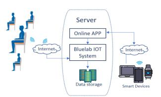
Figure 1. System configuration with the chair system being in contact with the server by wireless and can be accessed by smart devices through internet connection.
