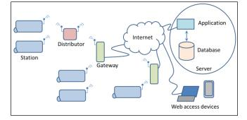
Figure 1. BlueLab's physical architecture.
