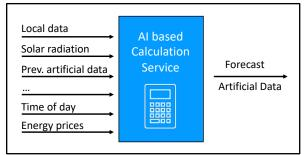
Figure 5 - Generator for Artificial Data
