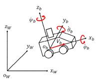
Figure 3. Notation related to vehicle motion.
