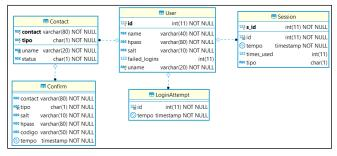
Figure 2. Database model for User access and authentication
