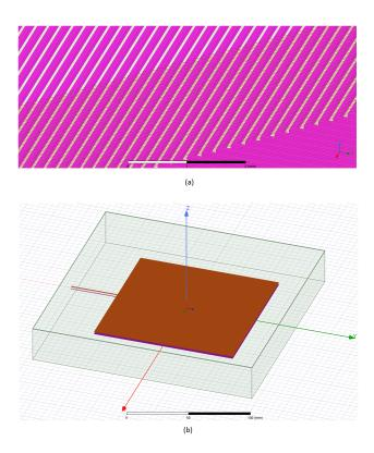
Figure 6. (a) Magnification of the 8 mH coils. Structure of the receiver (brown) and transmitter (purple) in the ANSYS analysis.
