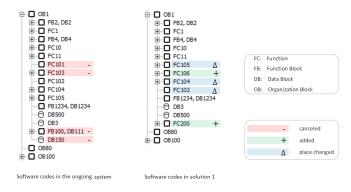
Figure 4. Comparison of software code in the PLC control system between the ongoing system and solution 1
