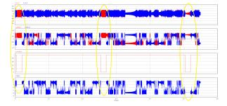
Figure 8. Time step of the chaotic behaviour when the receiver is disconnected (highlighted in yellow): the LC and memristor voltage  $V_{LC}$  and  $V_M$  in receiver and transmitter, respectively in blue and red. At the disconnection (in the  $3^{rd}$  graph), the receiver memristor holds its last status shown in the  $4^{rd}$  graph.
