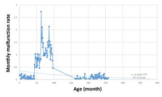
Figure 2. The average malfunction rate of the Wenhu Line central computers as s function of age (month).
