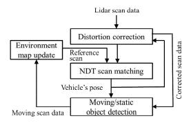
Figure 2. Overview of NDT-based SLAM.
