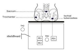
Figure 2. Seat sensors: PE1, PE2, and PD13 are pressure sensors, while TH1 and TH2 are temperature and relative humidity sensors.
