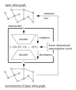
Figure 4. Traditional encoder-decoder approach.
