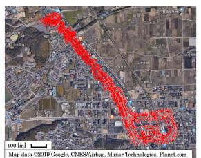
Figure 6. Point cloud map (top view)
