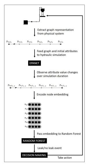
Figure 6. Process flowchart for training and executing machine.
