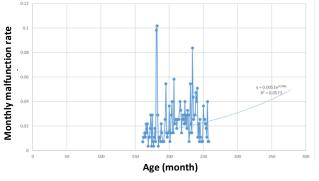
Figure 3. The average malfunction rate of the Muzha Line screen door as s function of age (month).
