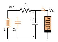
Figure 1. Memsistive circuit developed by L. Chua[10].
