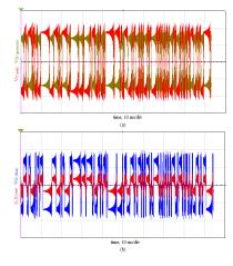
Figure 9. Time step of the chaotic behaviour in the receiver: the memristor voltage  $V_M$  in greenish and internal status  $V_0$  in red(a) and coil current  $i_L$  in red and memristor voltage  $V_M$  in blue (b).
