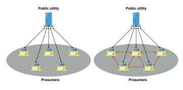
Fig 1. Present energy trading. Fig 2. Peer-to-peer energy trading.
