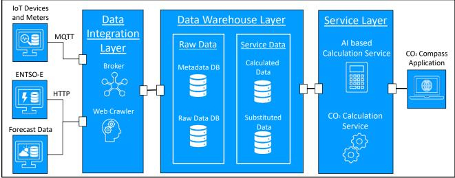
Figure 3 - Enhanced Architecture of the CO<sub>2</sub>-Compass
