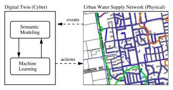
Figure 1. High-level representation for an urban water supply network digital twin (cyber) working alongside a physical urban water supply network.
