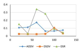
Figure 5. Average delay [sec] vs number of nodes, no DOS.
