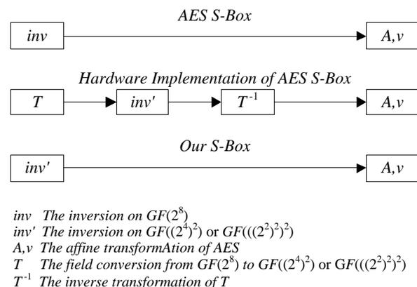
Figure 1. Structures of the different S-boxes in this paper.
