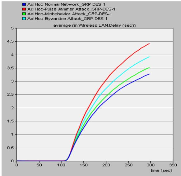
Figure 7. Delay results of the normal network with and without network attacks for GRP
