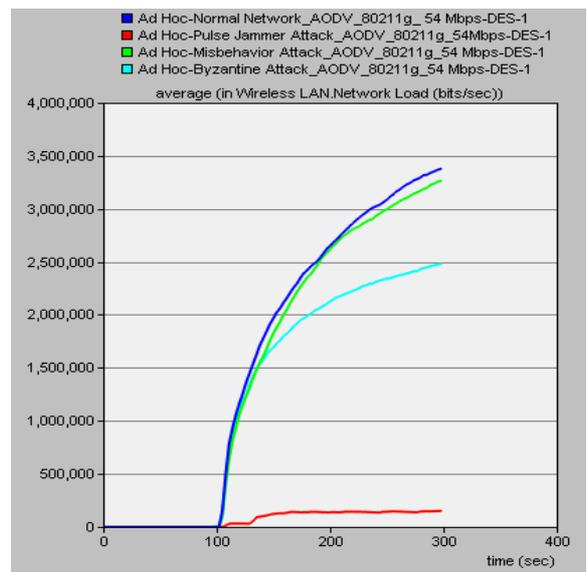
Figure 9. Network load results of the normal network with and without network attacks for AODV with respect to the IEEE 802.11g standard
