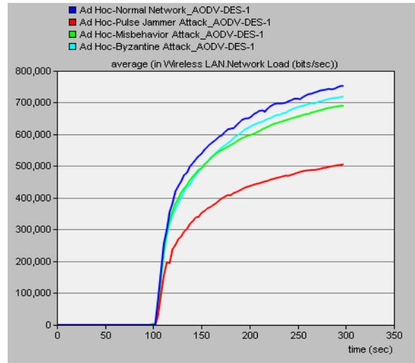
Figure 6. Network load results of the normal network with and without network attacks for AODV routing protocol
