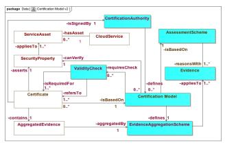
Figure 1: Model Based Certificates
