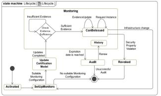
Figure 2: Life cycle of incremental certificates
