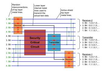
Figure 1. A regular active shield implementation with fixed interconnections.
