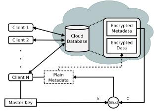
Figure 1. Cloud database architecture
