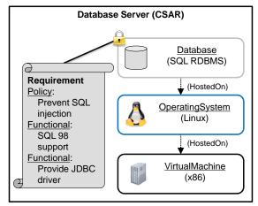
Figure 5. Transformation Example - Input Topology.
