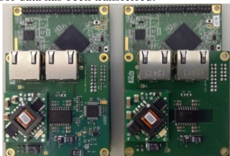
Figure 2: The photos of printed circuit boards of gateway (left) and sensor node (right).
