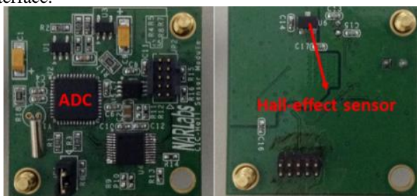
Figure 5: Top-view and bottom-view photos of the hall-effect sensor
