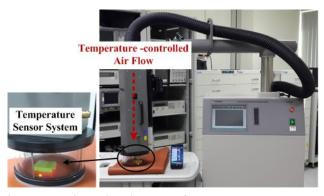
Figure 9 Experimental environment of a temperature sensor system.
