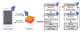
Figure 7 Communication flow path between smart phone and platform.
