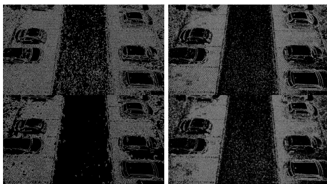
Figure 13. Two different edge detection algorithms tested with different parameters. From left to right, top to bottom: Canny Min=10, Max=50, Sobel X=1, Y=1, Canny Min=2, Max=200, Sobel X=2, Y=2.
