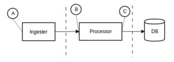
Figure 4. Graphical representation of the experimental methodology used to assess the performance of Chimera, tier by tier.
