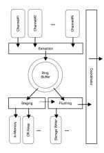
Figure 3. Processor internals. A ring buffer disciplines the interactions between producers and consumers, respectively the inbound channels receiving the data samples to process, and the staging and flushing sub-stages that store the data either for further processing or for durable persistence.
