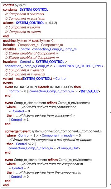
Figure 12. Composition of Component n and Component m machines.
