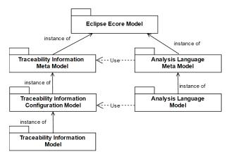
Figure 6. Conceptual Integration of Model Layers.
