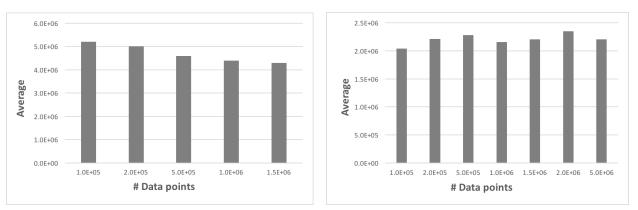
(a) Ring buffer stress test results. Synthetic traffic was generated as (b) Journaler stress test results. Synthetic traffic was as per ring buffer. messages of average size 500 Byte.
