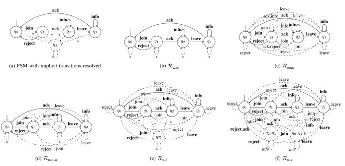
Figure 3. FSMs with states and transitions (dashed) added by the implicit error assumption (a) and different  $\mathcal{R}$  (b)-(f). **Bold** labels indicate an accepting, regular labels a rejecting, and *italic* labels an inconclusive verdict. The wild-card '\*' matches all events that have no other transition in the state.
