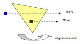
Figure 3. The application of Winding number method
