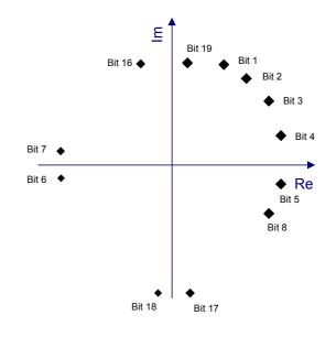
Figure 10. BPSK constellation of a received signal
