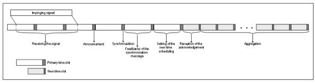
Figure 3. Time delay of the receive collaboration in TDMA based WSNs
