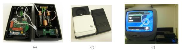
Figure 4. POBICOS-enabling real objects: (a) the RS232 adapter; (b) the power socket; (c) the TV set-top-box.
