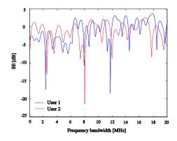
Figure 1. Magnitude of channel transfer function for a radio channel with multiptath.
