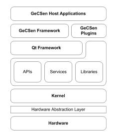
Figure 2. GeCSen on top of OS Architecture
