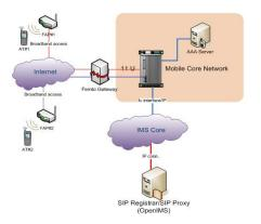
Figure 4. IMS-Femtocell integrated system architecture
