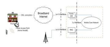
Figure 2. Logical architecture of LTE-based femtocell
