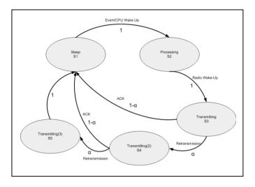
Figure 1.Simple Semi-Markov Chain model of event triggered operation
