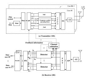
Figure 4. Proposed multiuser diversity OFDMA with frequency symbol spreading and adaptive subcarrier block selection.
