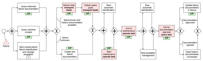
Figure 4 Context-aware workflow for handling a failure in the Smart Factory
