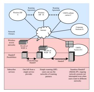
Figure 6: WLAN-UMTS Interworking (adapted from [12])
