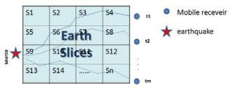
Figure 1. The discrete slowness model for seismic tomography.
