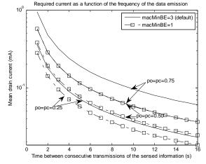
Figure 3. Mean drain current as a function of the frequency of data emission and two values of *macMinBE*. Power consumption due to reassociations not considered
