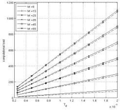
Figure 6. Effects of increasing L on the computational load for different values of M
