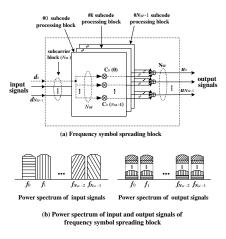
Figure 5. The structure of frequency symbol spreading block and power spectrum of input and output signals of frequency symbol spreading block.
