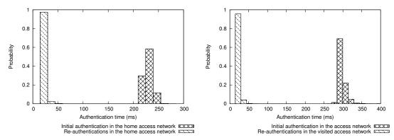
(a) EAP-Kerberos performance in the home access network (b) EAP-Kerberos performance in the visited access network
