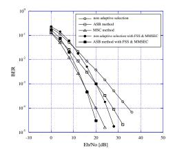
Figure 9. BER of non adaptive selection, the ASB method, the MSC method, non adaptive selection and the ASB method using frequency symbol spreading and MMSEC with 4 users and  $N_{SF}$ =16 for Doppler frequency of 10Hz.
