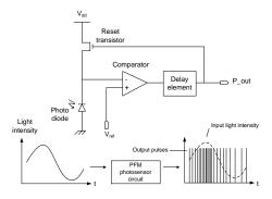
Figure 1. Architecture of PFM photosensor
