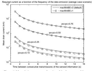
Figure 4. Mean drain current as a function of the frequency of data emission and two values of *macMinBE* (re-associations are considered)
