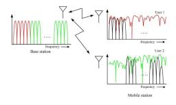
Figure 3. Resource allocation method with adaptive subcarrier block for each user.
