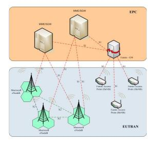
Figure 3. Logical architecture of LTE-A based femtocell
