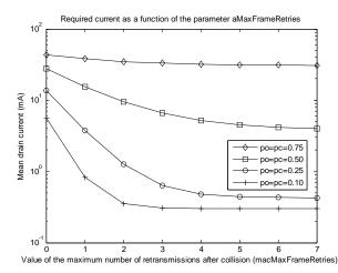
Figure 6. Mean drain current as a function of *macMaxFrameRetries* (rate=1 packet/s) (re-associations are considered)
