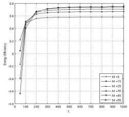
Figure 2. Effect of increasing the distance between remote and cooperating nodes on energy efficiency for different values of M
