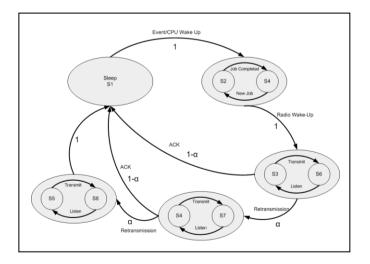
Figure 2.Semi-Markov Chain model with embedded chains
