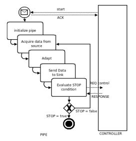
Figure 1. BPMN-like notation for a synchronous pipe from a source to a sink operation.
