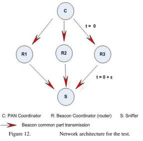
The receiver is in the transmission range of the PAN Coordinator and the three routers, i.e., the sniffer's software shows two frames which will allow us to measure the time offset between the reception and the transmission of the frame. When a router receives the frame from the PAN Coordinator, it retransmits it immediately. As it is shown in Figure 13, the sniffer receives two frames: the first one is the
