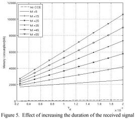
Figure 5. Effect of increasing the duration of the received signal on memory consumption
