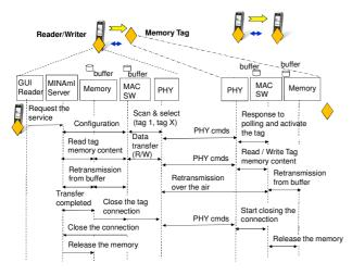
Figure 8. Basic MINAmI subsystem communication setup sequence
