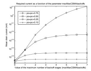
Figure 9. Mean drain current as a function of *macMaxCSMABackoffs* (rate=1 packet/s). Power consumption due to re-associations not considered
