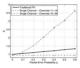
Fig. 8. Average Energy per packet as a function of the experienced packet error probability for frequency hopping and single channel scheme. Results are obtained considering N = 100 packets.
