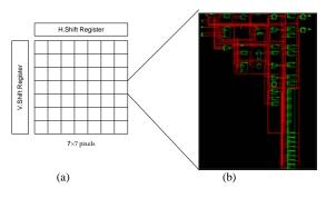
Figure 9. (a) Schematic diagram of an array, (b) RTL schematic per pixel
