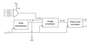
Figure 6. Block diagram of digital circuit per pixel.
