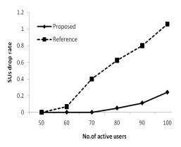
Figure 4. Sceduling unit drop rate Vs system load
