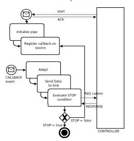
Figure 2. BPMN-like notation of an asynchronous pipe between a source and a sink. The callback endpoint is invoked when data can be consumed.
