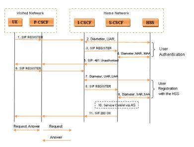
Figure 5. Signalling messages flow in registration procedure
