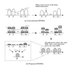
Figure 6. Power spectrum of the proposed OFDMA system.
