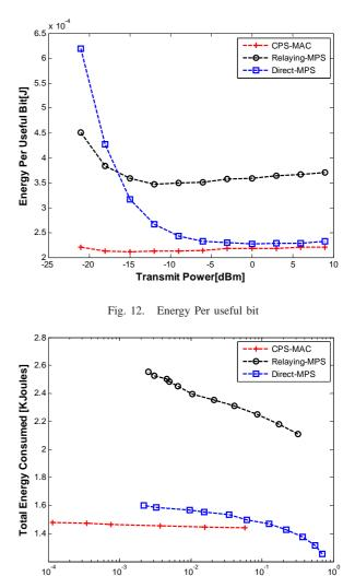
Fig. 13. Total Energy Consumed vs Packet Error Rate tradeoff
