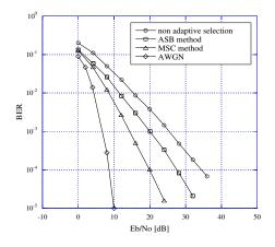
Figure 7. BER of non adaptive selection, the ASB method and the MSC method for multiuser diversity OFDMA system with 4 users and  $N_{SF}$ =16 for Doppler frequency of 10Hz.
