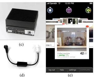
Figure 2. The hardware in the household consist of a sensor measuring the main meter in the fuse box (a), sensors that measure appliances; either off the shelf sensors (a) or custom made sensors (d), a base station (c) that receives the data from the sensors, controls the ambient interface and delivers data to the data storage. Next to real time consumption data is visible in the client user interface (e).
