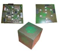
Figure 1. Smart Micrel Cube: on the top left the inner surface of the master face, with all the main components and on the top right the inner surface of
