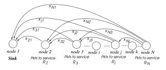
Figure 3. The linear network showing proportion of packets transmitted to different nodes towards the sink
