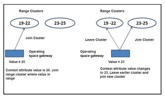
Figure 3. Joining and leaving of range clusters for OSG.
