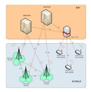
Figure 4. E-UTRAN Architecture including the deployment of Femtocell
