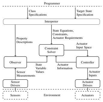
Figure 3. Architecture of the Runtime-Environment.
