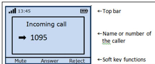
Figure 19. Ascom 9d24 prototype Incoming call (number)
