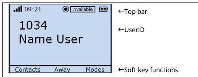
Figure 15. Ascom 9d24 prototype main screen
