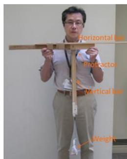
Figure 11. Protractor used in this research
