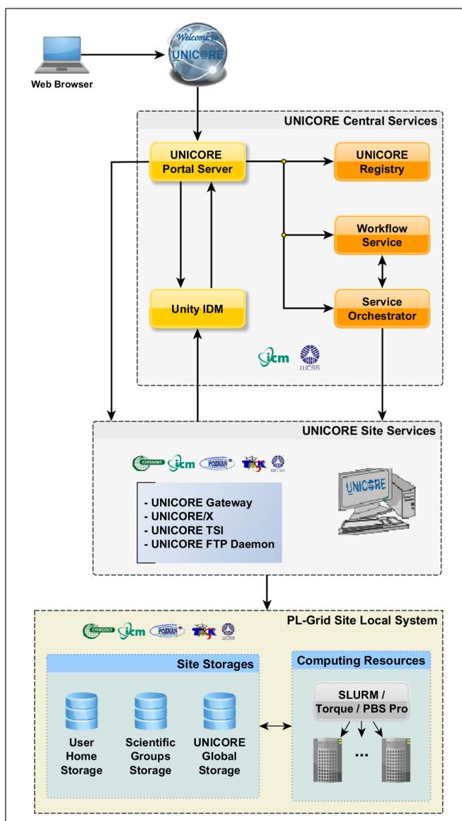
Figure 2. The UNICORE Portal Deployment in the PL-Grid.
