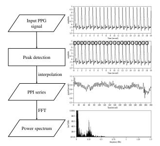
Figure 2. An example procedure of PRV.
