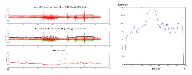
Figure 3: Data comparison for indexes computation: (a) raw signals and related offline processing with standard algorithms, (b) 5-sec average HR computed by WES system.
