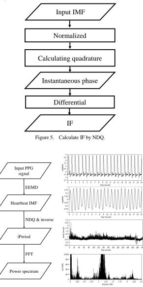
Figure 6. The procedure of iPRV.
