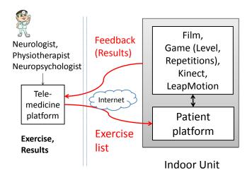
Figure 1. Head Platform Architecture.
