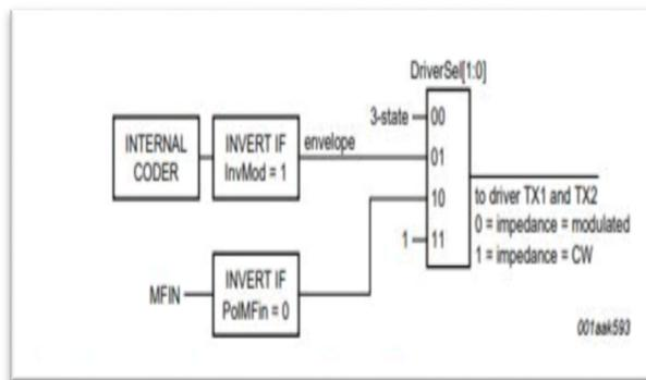
Figure 1. Serial Data Switch for p-driver Tx1 & Tx2 [8].
