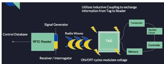
Figure 4. Access Control Systems - Component Information.
