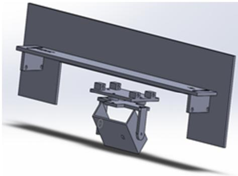
Figure 4. 3D model of the camera mount mechanism.
