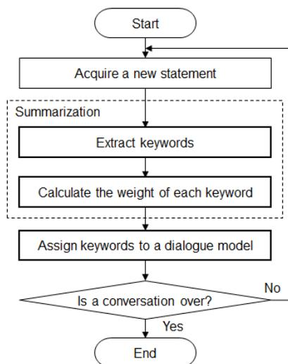
Figure 1. Process flow of the proposed method.
