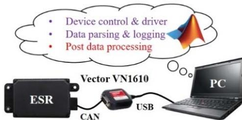
Figure 5. Radar measurement set-up.
