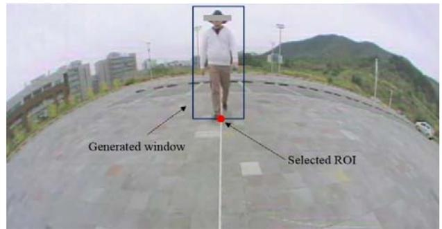
Figure 13. Example of ROI selection and window generation for the camera sensor
