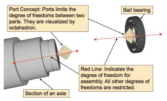
Figure 5. A port concept is used to assmble two virtual parts.
