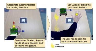
Figure 3. a) To translate a 3D model the user has to grasp an axis of the corrdinate system that appears above the 3D model, b) The user has to open his hand in order to release the 3D model.
