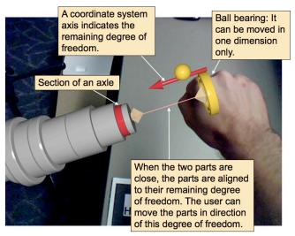
Figure 7. Second step of the virtual assembly. The user can only move the part in the remaining degree of freedom.
