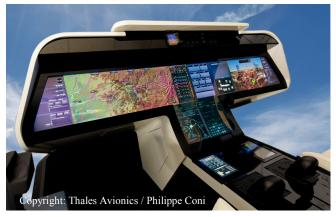
Figure 2. The ODICIS single-screen tactile cockpit.
