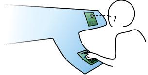
Figure 1. The "deported view" concept in a cockpit.
