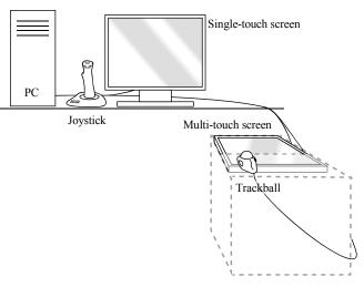
Figure 4. Illustration of experimental setup.
