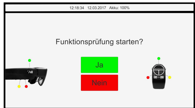
(a) Initial screen. The worker is informed about the key assignment and can start the functional check by pushing the touch-pad either on the HWD or on the finger-worn input-device.
