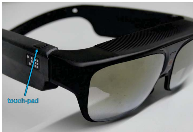
(a) Front of the ODG R-7 with the touch-pad. Between the lenses is the camera and above a flash-led.
