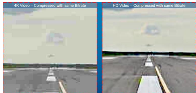
Figure 3. Artefacts in 4K vs Full HD compressed video streams with same pixel per degree resolution.
