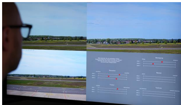
Figure 16. Test Subject conducting the perceived video quality evaluation task comparing three video streams out of the three cameras.
