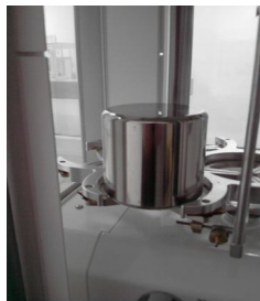
Fig.1. Reference standard of 1 kg, Ni81
