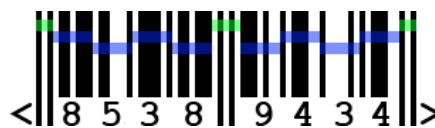
Figure 7. Structure of EAN-8 barcode, with the black-white-black pattern in the beginning, middle, and end.
