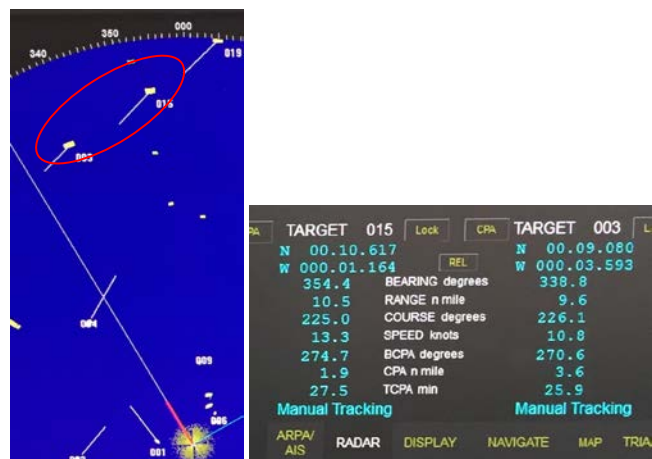
Figure 2. Radar plot showing current position and surrounding ships. Six ships are plotted (numbered and with lines) and details on 015 and 003 (the two circled ships) are illustrated to the right.
