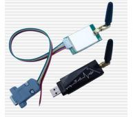
Figure 4. PLC Wi-Fi attachments (upper one for PLC, other one for PC)
