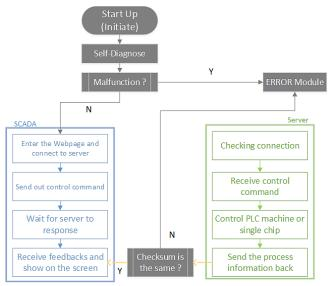
Figure 5. PLC's working process
