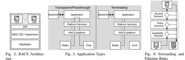
Two main categories of applications can be deployed at RACS servers, depending on the traffic flow: transparent/passthrough and terminating applications (cf. Fig. 3). The dotted line in Fig. 3 represents the control plane, which is available in both applications types. The line having arrowheads represents out-of-band communication that both application types are optionally able to perform. The solid line is the user plane.
