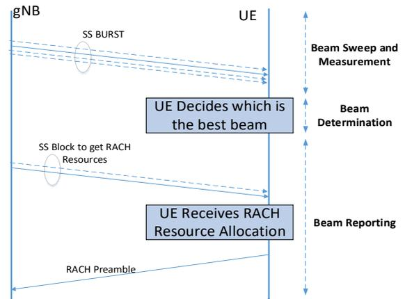
Figure 1. 5G Stand Alone beam management procedure
