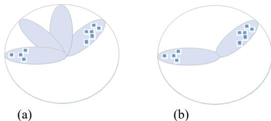
Figure 3. Beam Sweeping in Sparsely distributed UE Scenario
