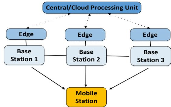
Figure 6. Deployment of ML/DL Algorithms at Wireless Edge
