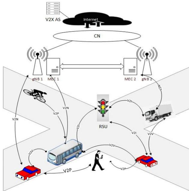
Figure 2. C-V2X Network Architecture with MEC and 5G
