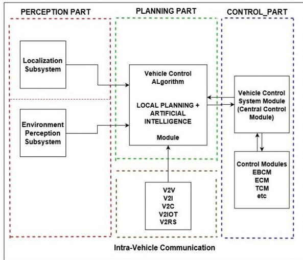
Figure 3. Overall Internal Architecture of Autonomous Vehicle.
