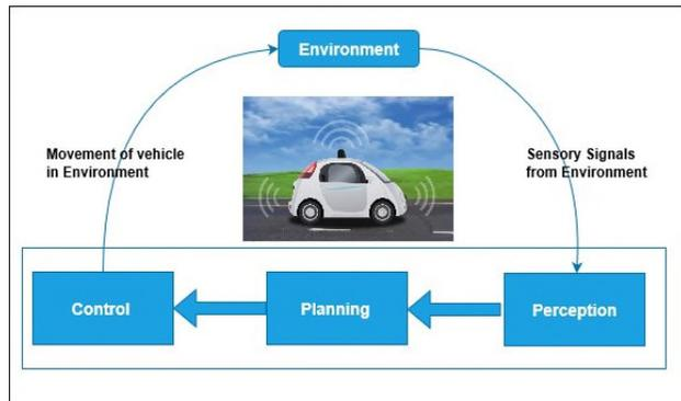
Figure 1. Major Systems of an Autonomous Vehicle.
