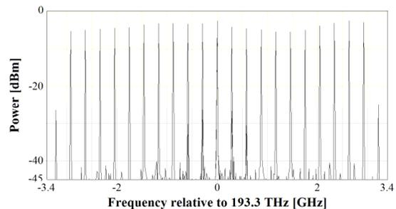
Figure 3. A spectrum of multi-wavelength optical frequency comb output.
