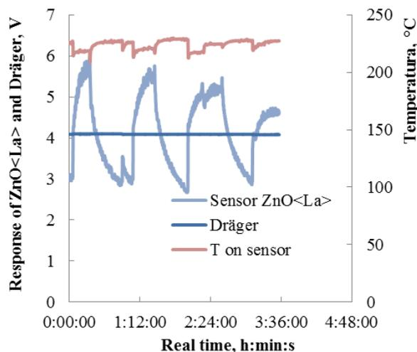
Figure 3. ZnO<La> sensors response to 10 ppm of H<sub>2</sub>O<sub>2</sub> vapours.
