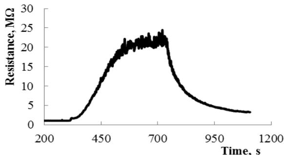
Figure 1. Resistance variation of the ZnO<La> sensor under the influence of 1800 ppm of H<sub>2</sub>O<sub>2</sub> vapours, work body temperature of 350 °C.
