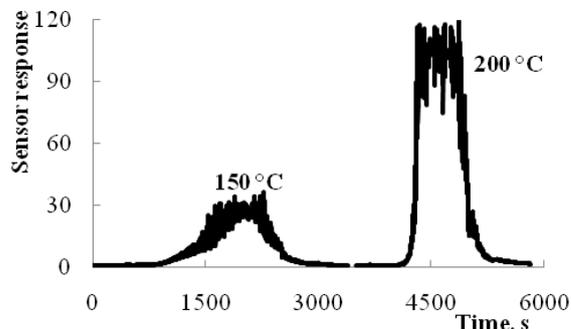
Figure 2. The SnO<sub>2</sub><Co> sensor response to 100 ppm of H<sub>2</sub>O<sub>2</sub> vapours at different work body temperatures.
