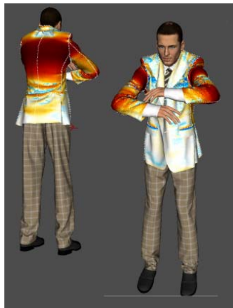
Figure 1. Garment simulation to result in strain values (colorcoded) with permission from [1].
