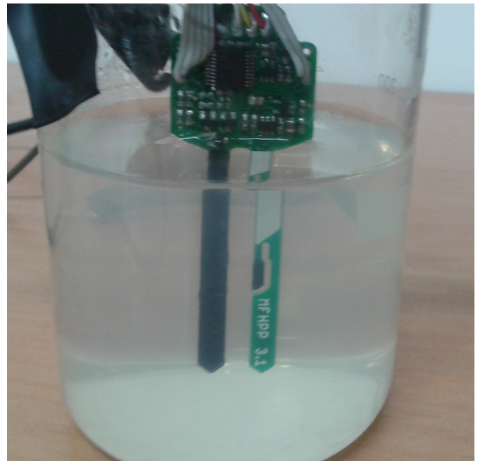
Figure 5. Probe distance calibration in agar solution
