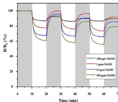
Figure 3. Response of sensor with  $P_{4,4,4,6}SPA$  to
