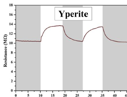
Figure 4. Response of sensor with  $P_{4,4,4,6}SPA$  to 10 ppm of yperite.
